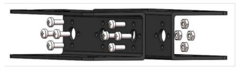
The beam is the base of the mechanical arm, which needs to be fixed on the bottom plate to prevent the mechanical arm from toppling.
